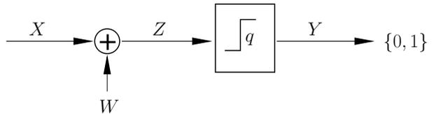
Fig. 1: The system model: some real input  $X$  is subject to additive noise  $W$  and is quantized with threshold  $q$  to yield binary output  $Y$ .
