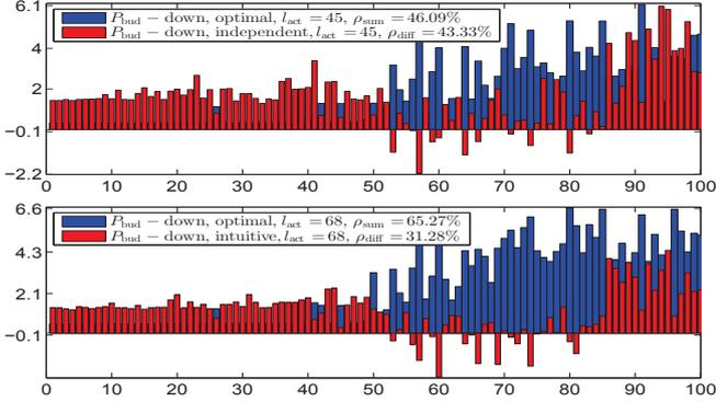
Fig. 5. Distribution of the SN power consumption is depicted for each SN index (x-axis) for ' $P_{\text{bud-down}}$ ' parameter set, see Table II.  $P_{\text{overall}} = 370.9$ . It is observed that the utilization of the intuitive pricing scheme in (13) enhances the network lifetime.
