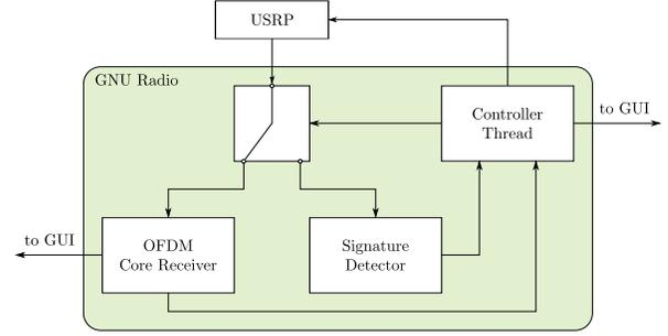
Figure 3: Receiver Architecture
