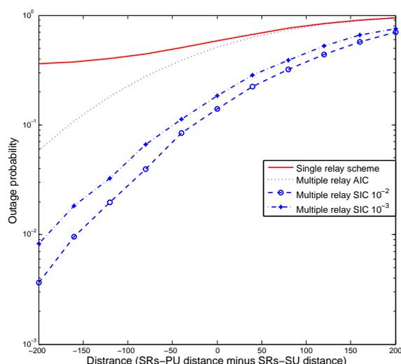
Fig. 4. The outage probability of the secondary transmission while the system topology is varied. The Packet size is set as 100 bits.
