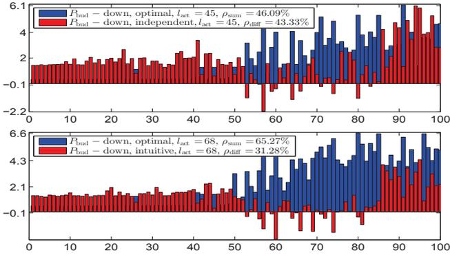
Fig. 5. Distribution of the SN power consumption is depicted for each SN index (x-axis) for ' $P_{\text{bud-down}}$ ' parameter set, see Table II.  $P_{\text{overall}} = 370.9$ . It is observed that the utilization of the intuitive pricing scheme in (13) enhances the network lifetime.
