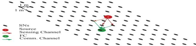
Fig. 3. The simulated SN setup, with 100 SNs on a surface. The source and FC nodes are positioned at the opposite sides, with 1 m distance from the surface. Each SN is positioned with 1 m distance to the adjacent node. A sub-set of SNs are active, at the depicted instance, to forward the sensed signal to the FC. The nodes at the center are better positioned compared to the nodes at the edge.
