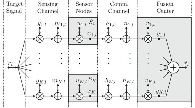
Fig. 2. System model of the distributed sensor network.
