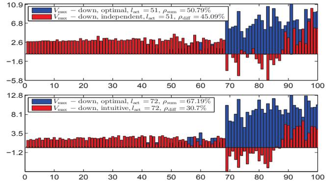
Fig. 8. Distribution of the SN power consumption is depicted for each SN index (x-axis) for ' $V_{\text{max-down}}$ ' parameter set, see Table II.  $P_{\text{overall}} = 516.8$ . It is observed that the utilization of the intuitive pricing scheme in (13) enhances the network lifetime.
