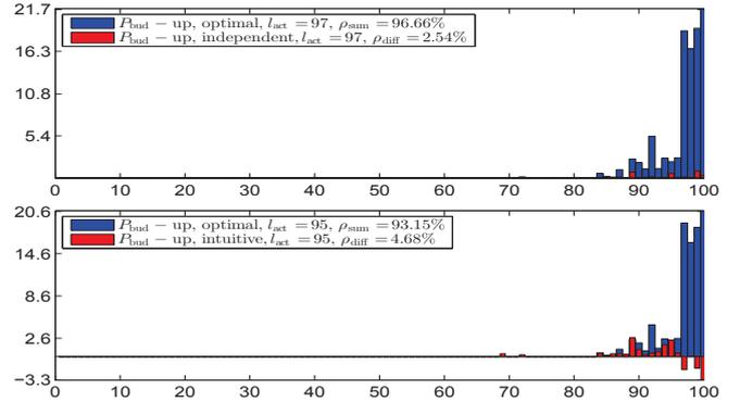
Fig. 6. Distribution of the SN power consumption is depicted for each SN index (x-axis) for ' $P_{\text{bud-up}}$ ' parameter set, see Table II.  $P_{\text{overall}} = 101.8$ . It is observed that the utilization of the intuitive pricing scheme in (13) reduces the network lifetime.
