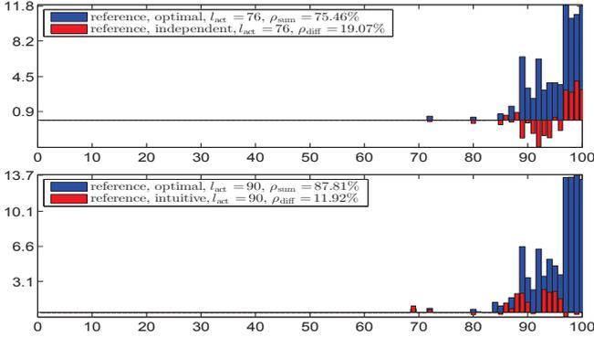
Fig. 4. Distribution of the SN power consumption is depicted for each SN index (x-axis) for 'reference' parameter set, see Table II.  $P_{\text{overall}} = 109.4$ . It is observed that the utilization of the intuitive pricing scheme in (13) enhances the network lifetime.
