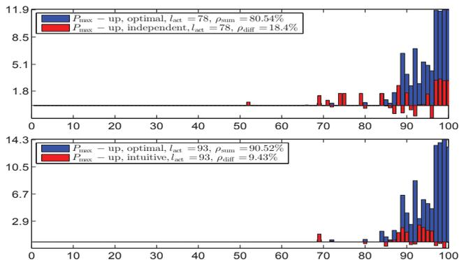
Fig. 10. Distribution of the SN power consumption is depicted for each SN index (x-axis) for ' $P_{\text{max-up}}$ ' parameter set, see Table II.  $P_{\text{overall}} = 108.8$ . It is observed that the utilization of the intuitive pricing scheme in (13) enhances the network lifetime.
