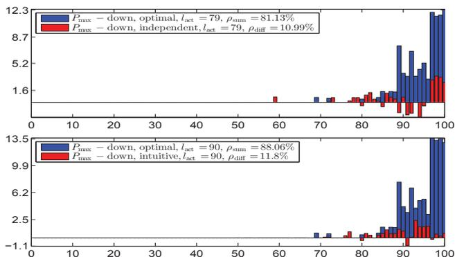
Fig. 9. Distribution of the SN power consumption is depicted for each SN index (x-axis) for ' $P_{\text{max-down}}$ ' parameter set, see Table II.  $P_{\text{overall}} = 115.6$ . It is observed that the utilization of the intuitive pricing scheme in (13) enhances the network lifetime.
