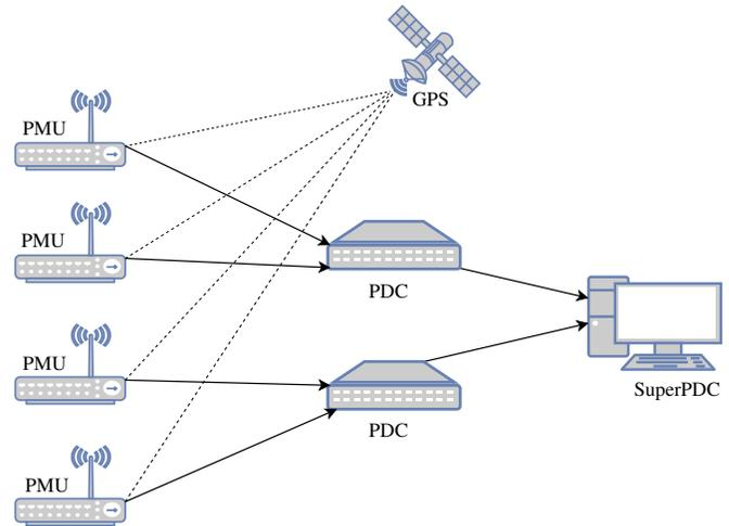
Fig. 1. Hierarchical network architecture of WAMS. PMUs send the phasor measurements, timestamped by the GPS signal, to SuperPDC over intermediate node PDCs
