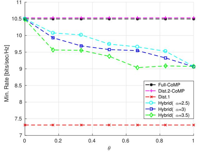
Fig. 2. Min. User Rate vs. Cooperation Threshold. Less cooperation reduces the minimum user rate performance, as cell edge users suffer.
