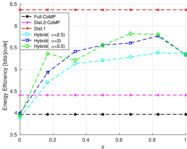
Fig. 5. Energy Efficiency vs. Cooperation Threshold. All the hybrid schemes are able to outperform full cooperation due to better quality associations.
