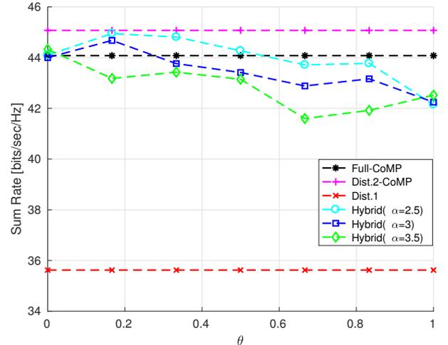
Fig. 3. Sum Throughput vs. Cooperation Threshold. The hybrid strategies do not experience a significant decline with higher threshold and are even able to outperform full cooperation due to better use of the limited backhaul resources.
