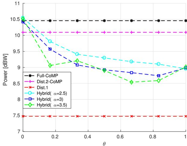
Fig. 4. Power Consumption vs. Cooperation Threshold. The power consumption generally reduces with less cooperation.
