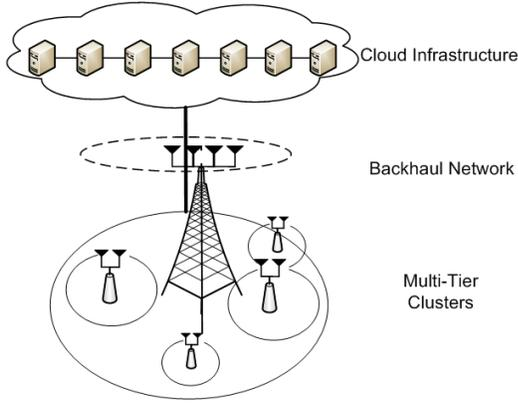
Fig. 1. Schematic of a heterogeneous network with cloud data center.
