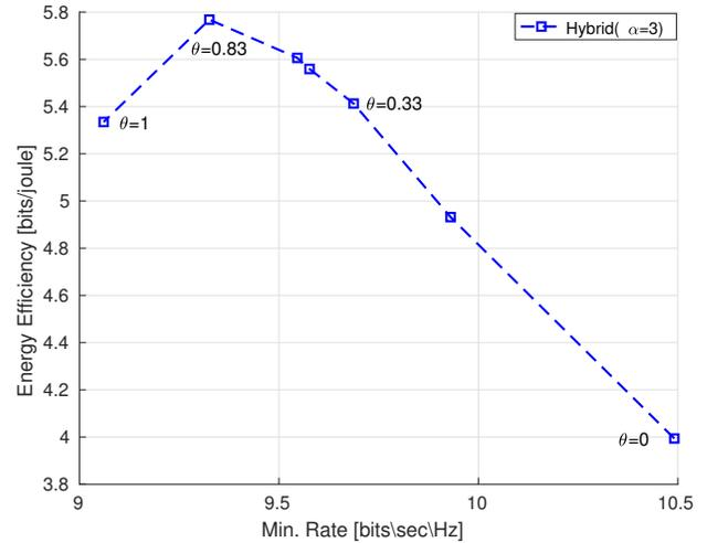
Fig. 6. Energy Efficiency vs. Min. User Rate, for case  $\alpha = 3$ . A good region of operation can be achieved based on two criteria when  $\theta = 0.83$ .
