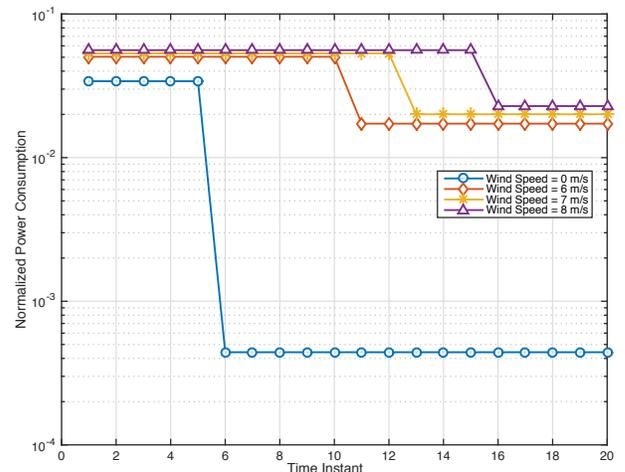
Fig. 7. Power consumption in function of wind speed.
