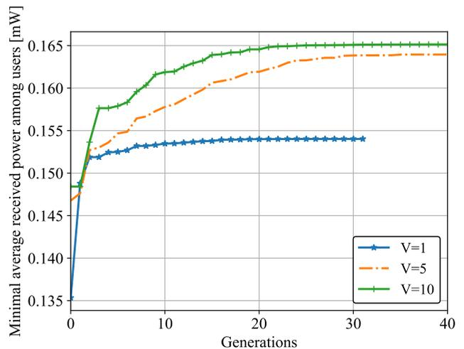
Figure 2. Convergence behavior of the proposed iterative algorithm for various maximum flying speed  $V$ .
