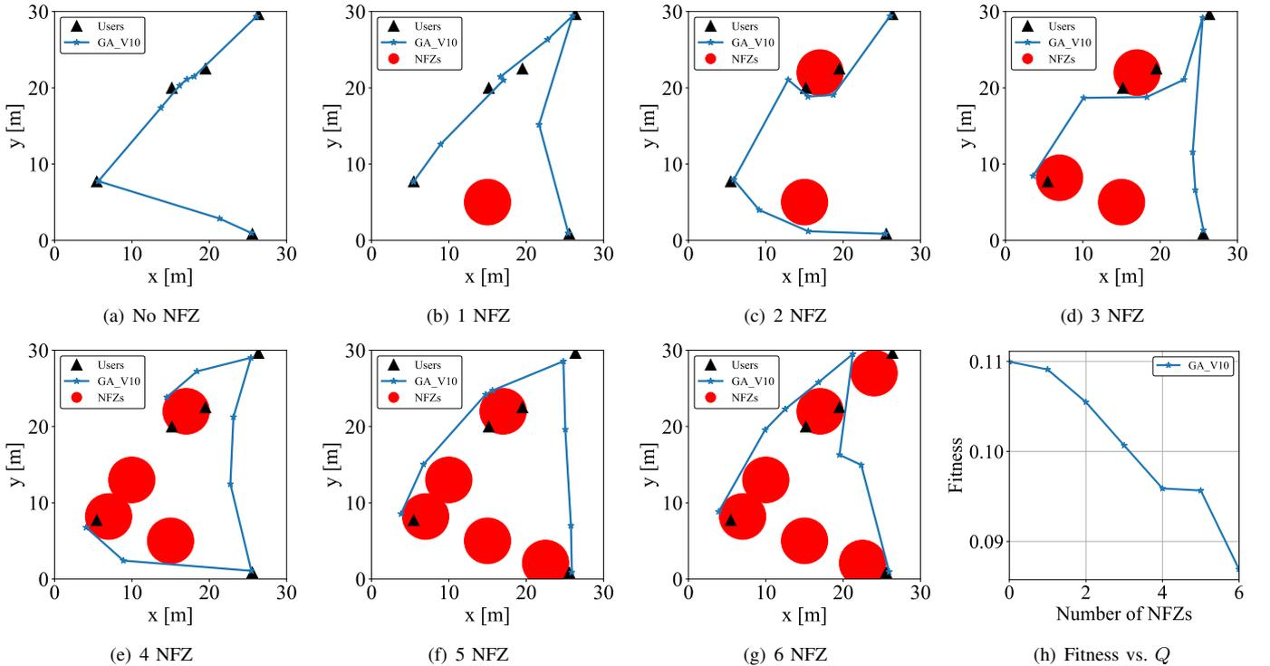
Figure 5. GA based trajectory design for various number of NFZs.
