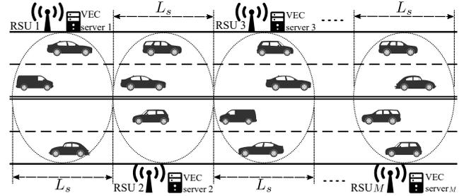
Figure 1. Illustration of the studied multi-lane bidirectional VEC network.
