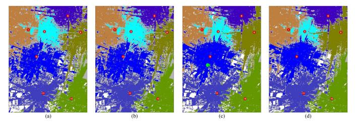
Fig. 10. CCO-related eNB cell footprints while handling coverage problems (switched off eNBs) and capacity problems (traffic hotspot). (a) Switched off eNBs cause coverage holes (white spaces). (b) Remaining eNBs predominantly compensate the degraded network coverage. (c) Reconfiguration with respect to a temporary traffic hotspot (bunch of spots below eNB 4). (d) Combination of coverage- and capacity-triggered reconfiguration.
