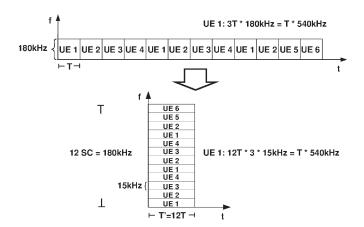
Fig. 7. Modeling scheduling over time by subcarrier allocation.
