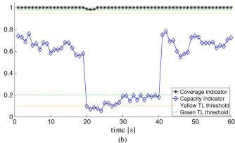
Fig. 9. Second-wise evaluation of the (upper) coverage indicator and the (lower) capacity indicator at the eNB (4) that is most affected by the traffic hotspot. The traffic hotspot is active from 20 to 40 s. (a) eNBs apply default configurations. (b) eNBs apply configurations according to CCO results.
