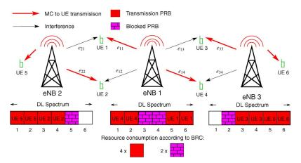
Fig. 1. Exemplary PRB allocation at eNBs and approximation of resource consumption for eNB 1.
