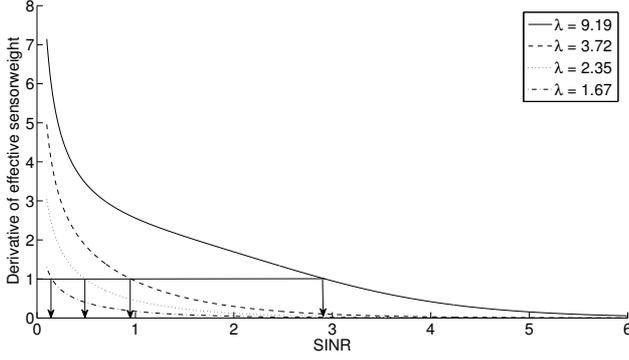
**Fig. 4.** Derivative  $\partial\tilde{\lambda}/\partial\gamma$  of the effective sensor quality  $\tilde{\lambda}$  with respect to the SINR  $\gamma$ . Here, the threshold  $\varrho$  is chosen to be equal to 1.
