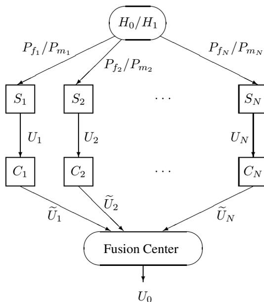
Fig. 1. Parallel fusion network with noisy channels.
