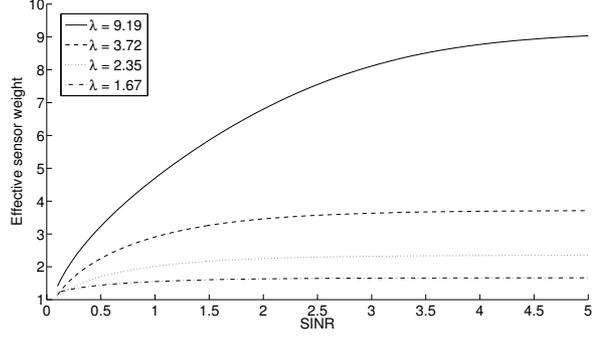
**Fig. 3.** Effective sensor quality  $\tilde{\lambda}$  as function of the SINR  $\gamma$  for different values of the initial sensor quality  $\lambda$ .
