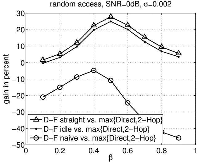
(b) Throughput improvement for the three Decode-and-Forward protocols. Throughput  $C_{df}$  (12) developed in Section III is compared to the conventional approach which consists of selecting the scheme Direct-Link or Two-Hop with highest throughput (11). The values are numerically calculated for  $SNR = 0.5$  decibels,  $\sigma = 0.002$ , and  $\gamma = 2$  following the procedure of Section IV.
