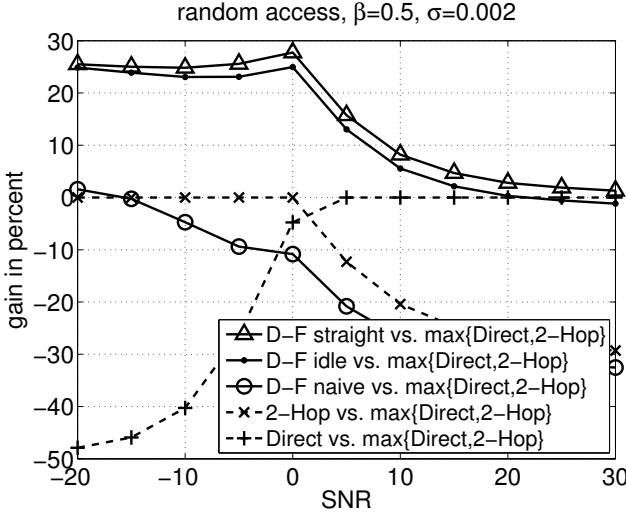
(a) Throughput improvement for the three Decode-Forward protocols. Throughput  $C_{df}$  (12) developed in Section III is compared to the conventional approach which consists of selecting the scheme Direct-Link or Two-Hop with highest throughput (11). The values are numerically calculated for  $\beta = 0.5$ ,  $\sigma = 0.002$ , and  $\gamma = 2$  following the procedure of Section IV.
