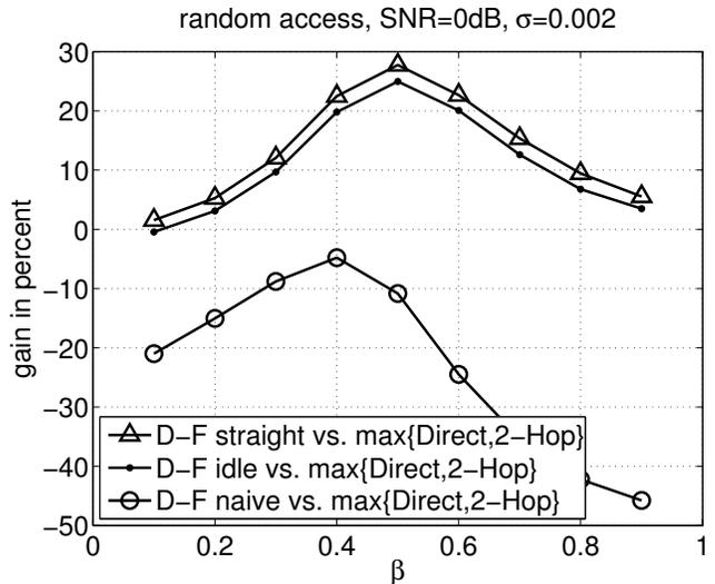
(b) Throughput improvement for the three Decode-and-Forward protocols. Throughput  $C_{df}$  (12) developed in Section III is compared to the conventional approach which consists of selecting the scheme Direct-Link or Two-Hop with highest throughput (11). The values are numerically calculated for  $\text{SNR} = 0.5$  decibels,  $\sigma = 0.002$ , and  $\gamma = 2$  following the procedure of Section IV.
