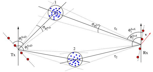
Fig. 4. MIMO multi path transmission with two clusters
