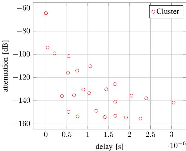
Fig. 6. Example of delay spread for clustered paths
