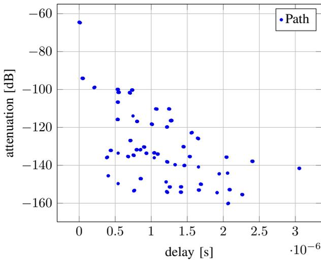
Fig. 5. Example of delay spread for paths generated by PIROPA
