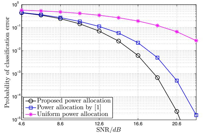
Fig. 2. Comparison of the proposed power allocation and a uniform power allocation in a network without power-limitation of the sensor nodes.
