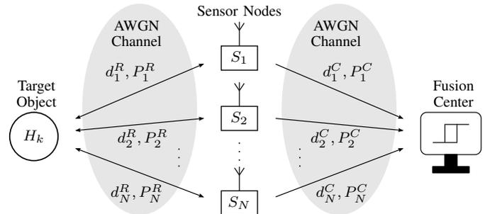
Fig. 1. System model of the distributed wireless sensor network.
