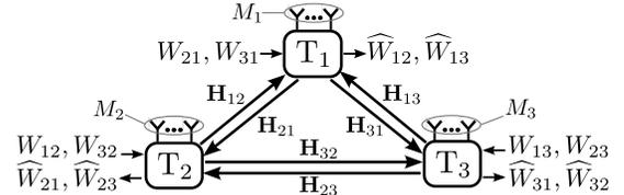
Fig. 1. The MIMO 3-way channel (or  $\Delta$ -channel) with  $M_i$  transmit and  $M_i$  receive antennas at each user  $T_i$ , with  $i = 1, 2, 3$ .
